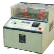
Automatic Oil BDV Test Set upto 120 kV
