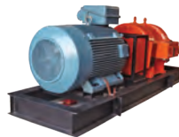
High-Voltage, High Frequency Test Set upto 10MVA
