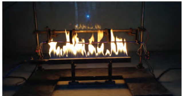
Fire survival – Cat CWZ Set Up
