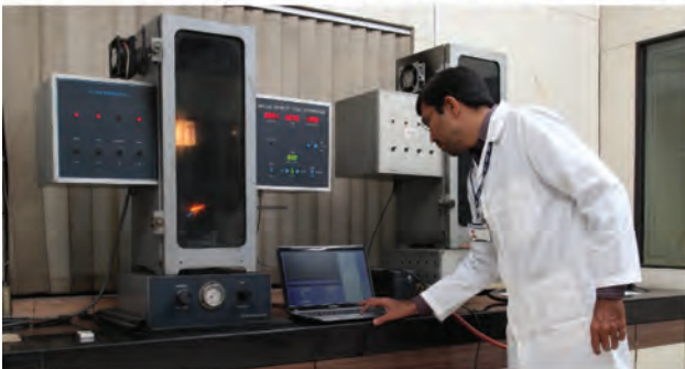
Smoke Density Testing in progress
